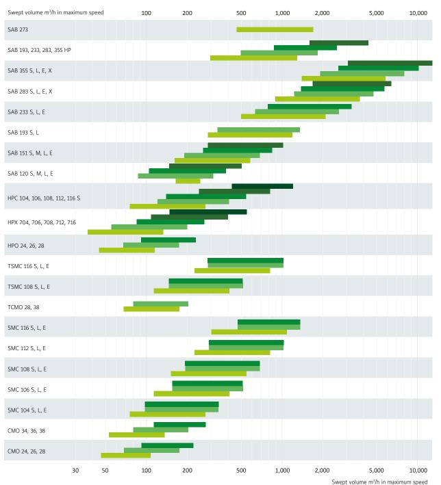
(Reciprocating compressors at 50/60 Hz. Screw compressors at 50/60/70/100 Hz)
